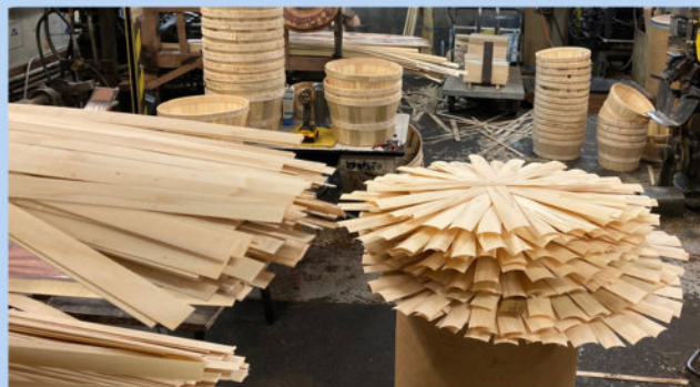
At Greenfield Basket, tulip poplar logs are loaded into a veneer lathe (left) to make thin sheets, which are cut into strips (above), and woven into baskets.
