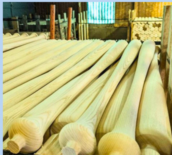
Below: Billets have been turned into rough bats at Larimer and Norton's mill. Photo by Warren County Visitors Bureau.
