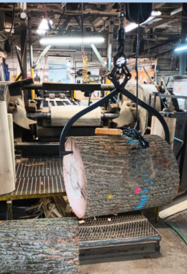
At Greenfield Basket, tulip poplar logs are loaded into a veneer lathe (left) to make thin sheets, which are cut into strips (above), and woven into baskets.
